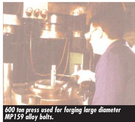
600 ton press used for forging large diameter MP159 alloy bolts.
