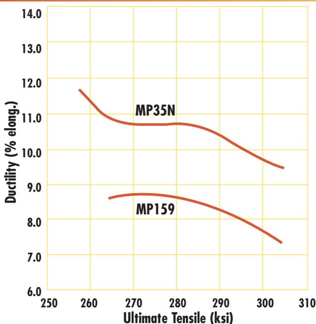
This graph details the high levels of ductility exhibited by MP35N and MP159 over their typical strength range. The combination of high strength and toughness is an important factor for fastener design.
