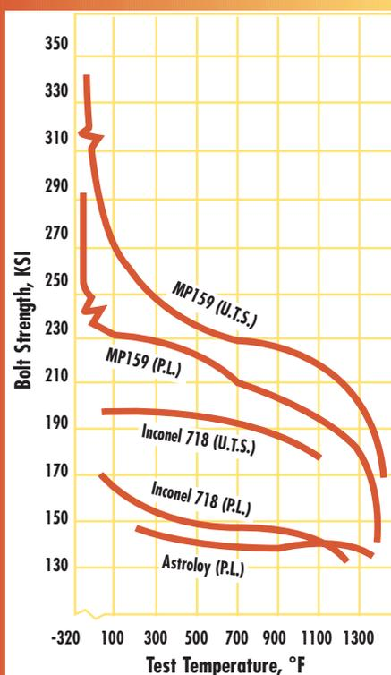
MP159 provides high yield and ultimate tensile strengths from cryogenic temperatures up to 1100°F.
