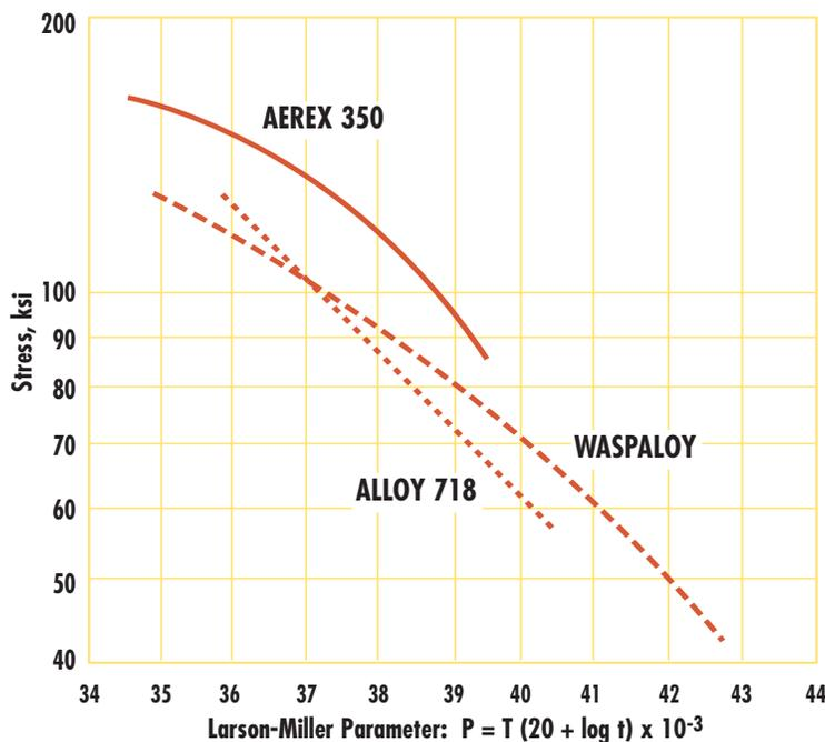
Stress rupture data are typically plotted in a Larson-Miller format, which allows the three parameters of stress, temperature and time to be evaluated. The curves presented plot the combination of these three variables necessary to produce rupture in specimens. Stress rupture resistance increases towards the upper right quadrant.
